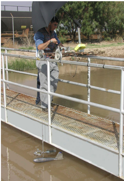
Water flow measurement in the Franklin Canal, El Paso, Texas
